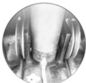
Dual hydraulic cylinders
